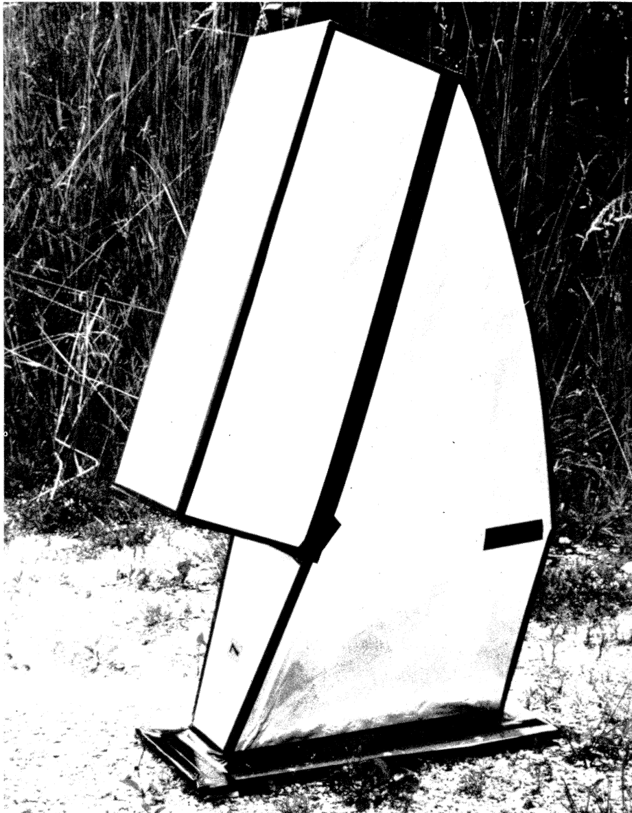
A futuristic-looking module of the silica aerogel detector built by a Brussels/Mons/Stockholm collaboration for use in the European Hybrid Spectrometer at CERN.
